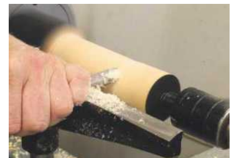
▲ Pic.15 One little tip when doing a planing cut is to control the tool by sliding your little finger along the toolrest; this will control the depth and direction of the cut
